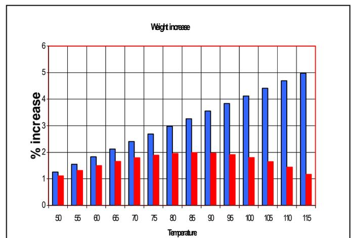
The conclusion is: With conditioning temperatures of 100 °C the weight increase will be initially up to +4,3 % (!). However, after a cooling period of 20 minutes the
